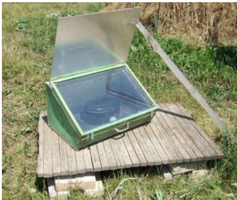
Simple but effective solar cooker, reaches boiling in an hour, and stays there as long as you like. Excellent for beans and pulses. Boiling water is a piece of cake.
